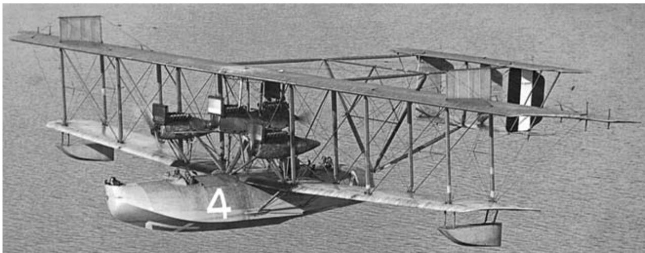
*A rare photograph of NC-4 during flight operations. NC-4 had three forward facing tractor engines and one center-mounted pusher engine. (Courtesy of the U.S. Navy)*
